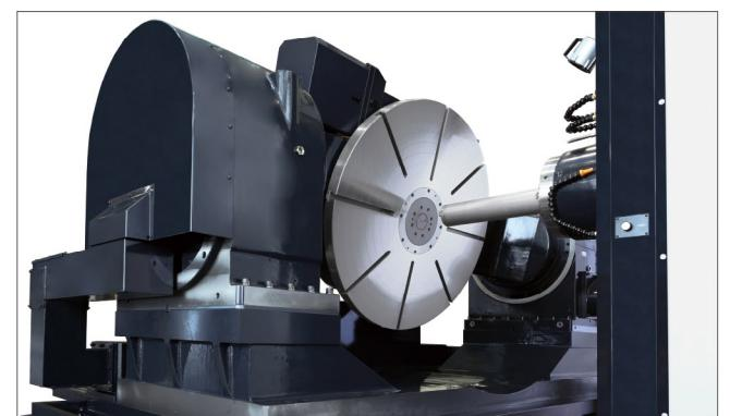
The boring spindle is, even without any tool attached to it, extendable to the table center.
